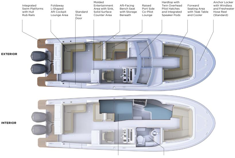
Port Side Cabin with Fore and Aft Six-Foot-Long Berths, Portlight, Overhead Vent, and Optional Air Conditioning Starboard Side Dedicated Head Compartment with Electric Freshwater Toilet
